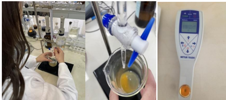
Fig4. Determination of total acidity
