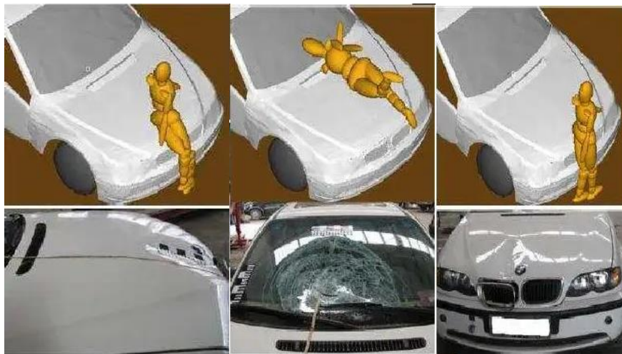
Figure 3. Vehicle damage in a collision with a pedestrian at 60 km/h.
