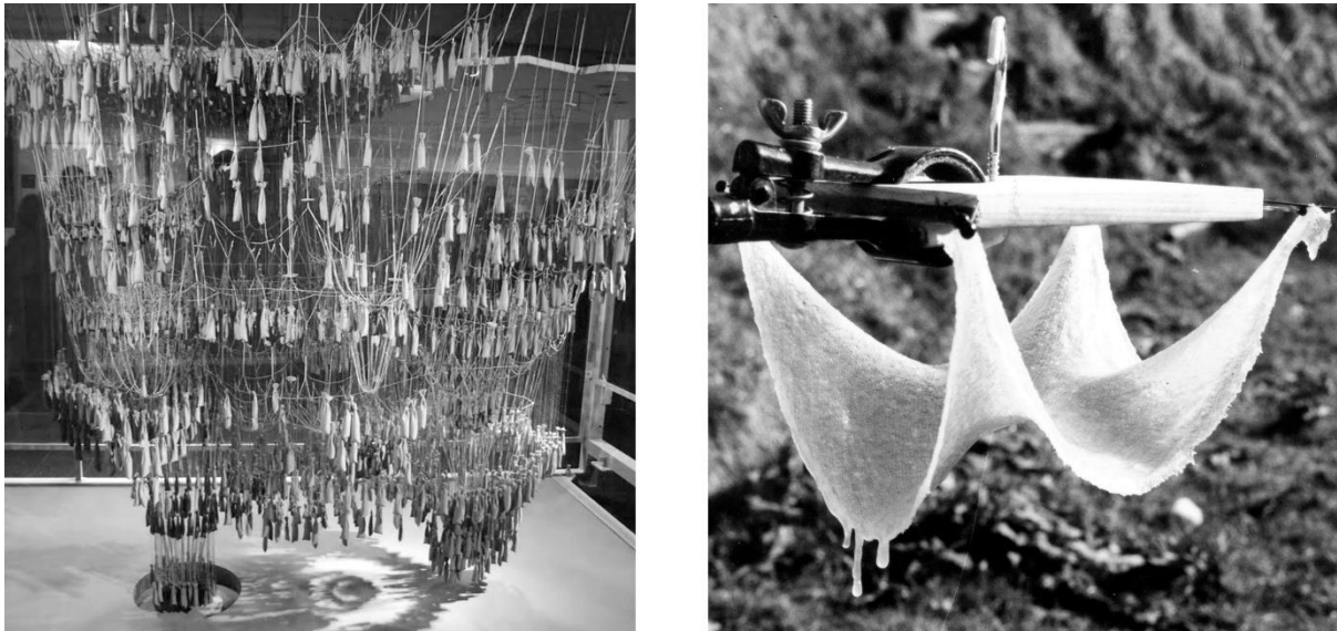
Figure 16. Reproduction of Gaudí's hanging chain model for the crypt of Colonia Güell, Barcelona (left); Form-finding using fabric and polyester by Heinz Isler (right)
