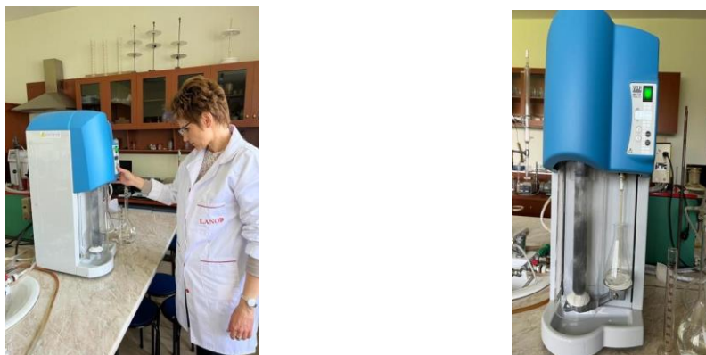
Figure 4 a) and b): Distillation process of samples (a) and Klejhdahl still (b).
