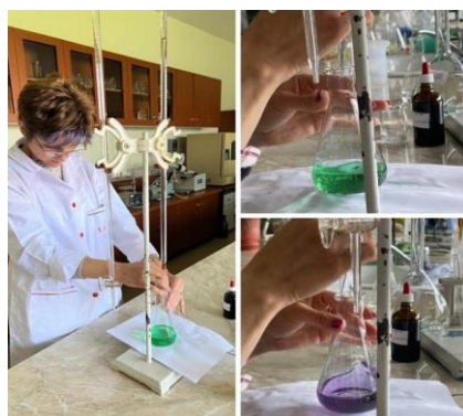
Figure 5: Moment of titration of samples, transition from green color to purple color
