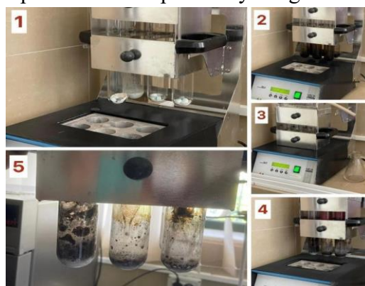
Figure 3: Protein mineralization process in a mineralizer with 6 parallel samples
