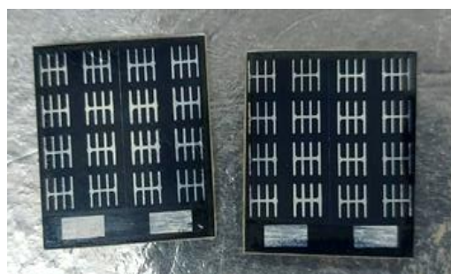
Figure 2. Two PV-cells, incorporating undoped CZTS and CZTS:Li absorbers, with front Ag-electrodes (fishbone-grid).
