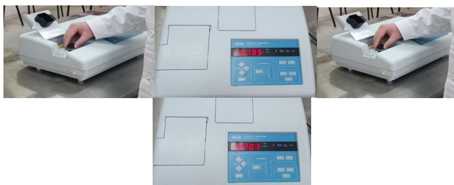
Figure3. Determination of Turbidity in sample W 1 and W 2
