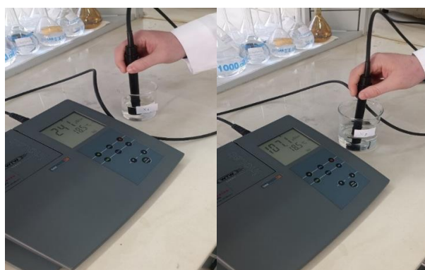
Figure2. Determination of Electrical conductivity in sample W 1 and W 2
