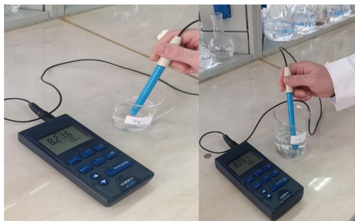
Figure1. Determination of pH in sample W 1 and W 2
