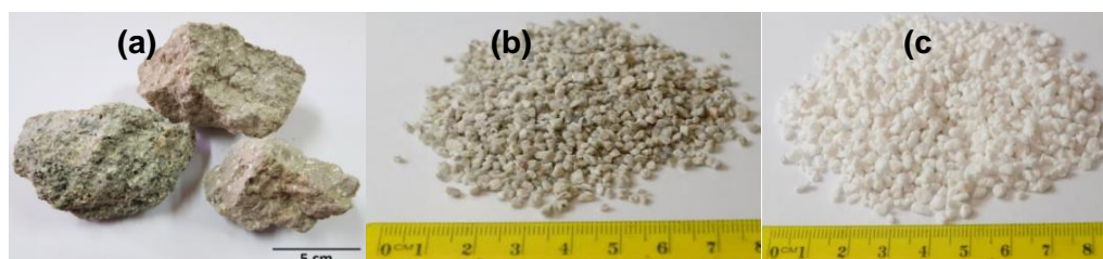
Figure 1. Perlite as seen (a) in a rock form collected from the Mariovo region, North Macedonia, (b) as an ore and (c) in expanded form, both supplied by the company Ausperl Pty Ltd.
