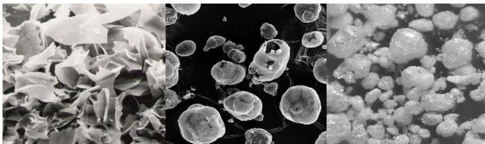
Figure 5. SEM images showing perlite as flakes, microspheres and bubbles [2] .
