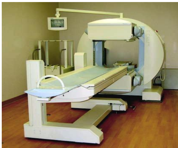
Figure 2. Conventional dual-head gamma camera system installed in 2009, used for planar scintigraphic imaging in nuclear medicine. Courtesy of the Department of Nuclear Medicine, University Clinical Center of Kosovo, Prishtina.
