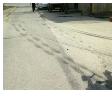
Figure 11 and 12. Traces of braking of the rear wheels of the towing vehicle under conditions of a blocked regulator of maximum brake force
