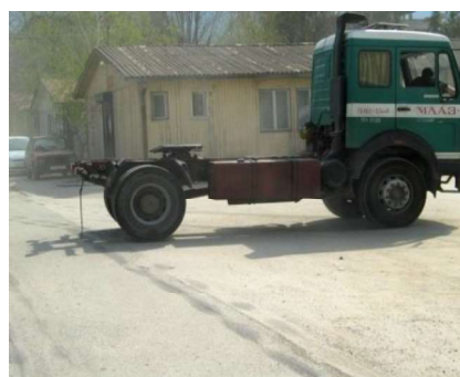
Figure 11 and 12. Traces of braking of the rear wheels of the towing vehicle under conditions of a blocked regulator of maximum brake force
