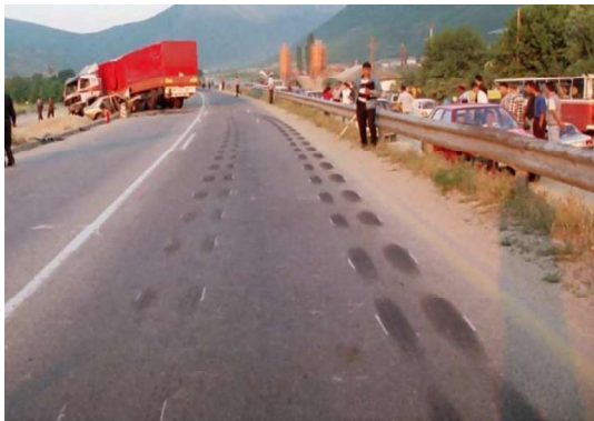
Figure 14. Traces of braking of the rear wheels of the towing vehicle while moving the towing train in a bend
