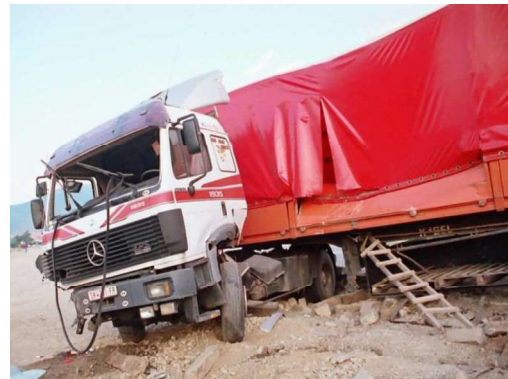
Figure 15. Disengaging of the towing train in the articular connection
