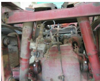
Figure 10. ASR device blocked in upper position under maximum brake pressure
