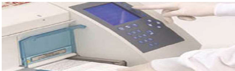
Figure 2. Vidas mini apparatus - apparatus for measuring immunoglobulins - immuno essey method (Albimedika Laboratory - Tetovo)
