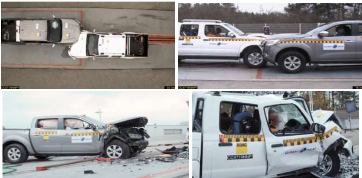
Figure 3. Crash test of new vehicle NISSAN NP300 Hardbody and used NISSAN NAVARA NP300
