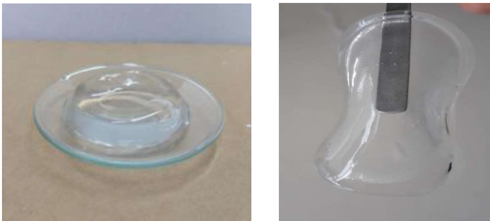
Figure 1. Alginate hydrogels obtained by polymerization of alginates with Ca^{2+} ions
