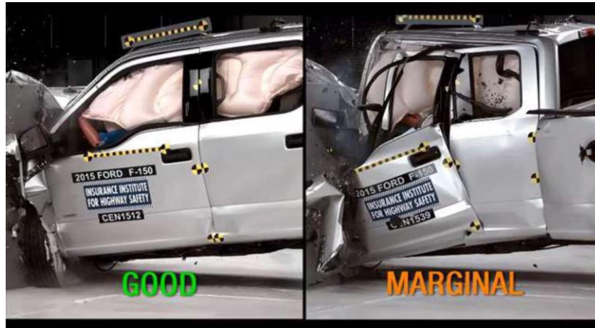
Figure 1. The condition of the passenger cabin after a head-on collision [2]
